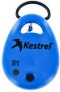
Know your temperature conditions anywhere with the small, rugged Kestrel DROP D1 Temperature Logger.
