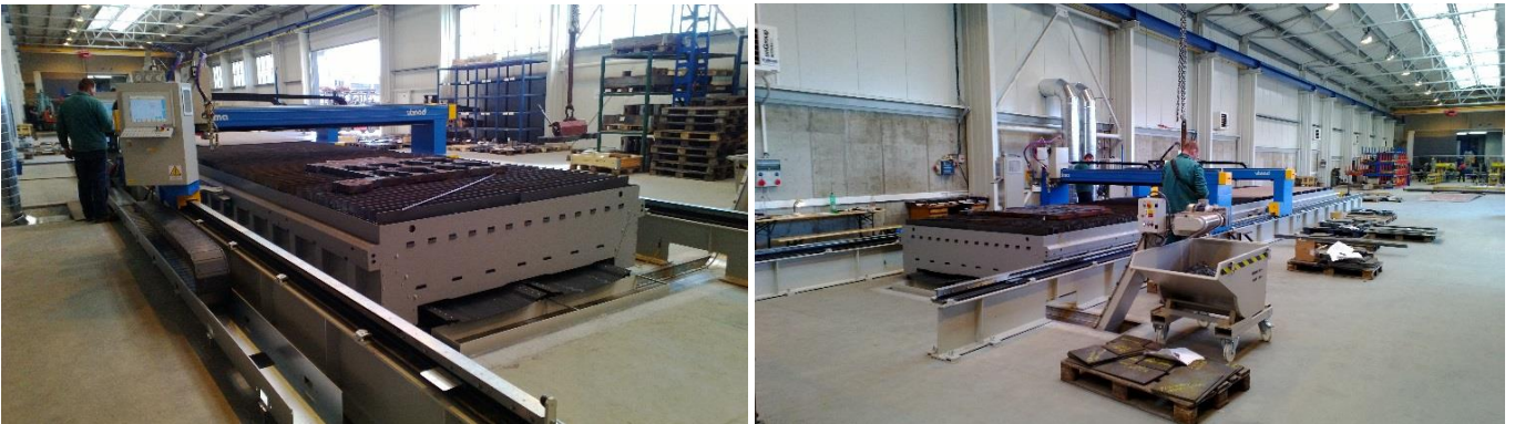
CNC Vanad PROXIMA, dimensions 35/60 with Hypertherm Powermax 125 plasma s., delivered in November 2015
