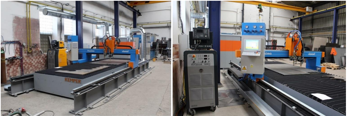
CNC Vanad PROXIMA, dimensions 30/170 with two portals, the KemTab Vibro extraction table with automatic discharge system, with Kjellberg HiFocus 440i plasma system, delivered in July 2013
