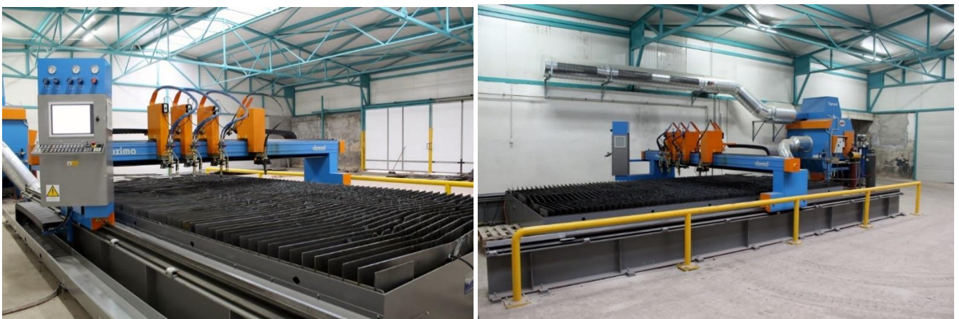
CNC Vanad PROXIMA, dimensions 35/60 with Hypertherm Powermax 125 plasma s., delivered in November 2015
